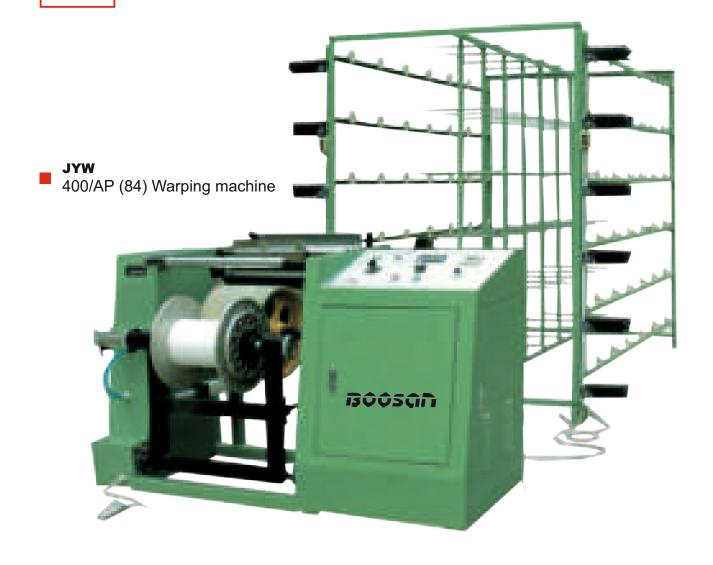
Optimally and flexibly used in the warping of kinds of nylon, faber, cottonyarn and etc
